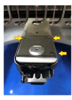
3. Remove the retaining finger by loosening one of the flat-head screws and removing the other completely to swing it off to one side (illustrated below)
