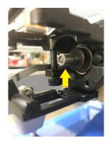
b. If the sleeve is stuck to the shaft and you are unable to take it off with your hand, use a pair of dykes and squeeze them on the seam where the sleeve meets the shaft in order to remove it without damaging your machine.
