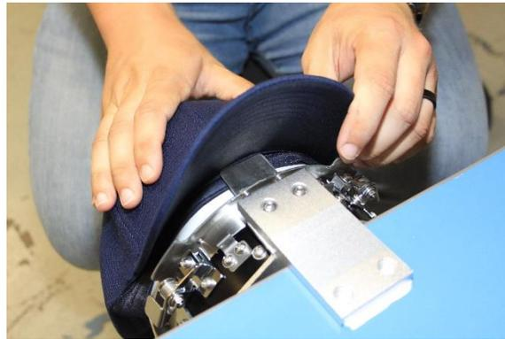
9. Placing one hand on the top of the cap, ensure that the sides of the cap are flat and that the black posts on the cap frame are inside the cap.
