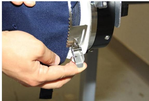
14. Pull each side of the cap down tightly around the outside of the black post at the bottom of the cap driver. Then, place one of your binder clips around the fabric and post. Do this on both sides.
