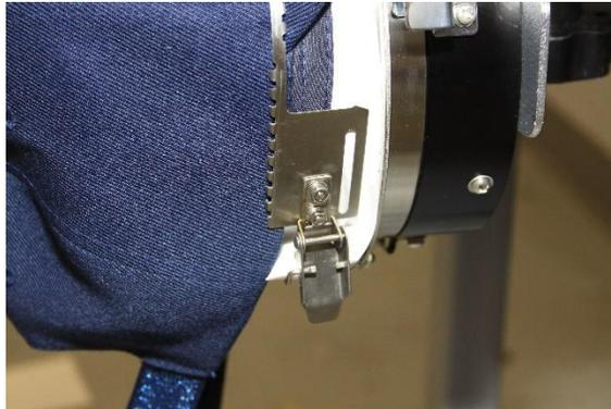
12. Looking at the metal alignment tab, move the center seam of the cap slightly to the left so that when you close down on the metal strap the cap centers itself on that tab
