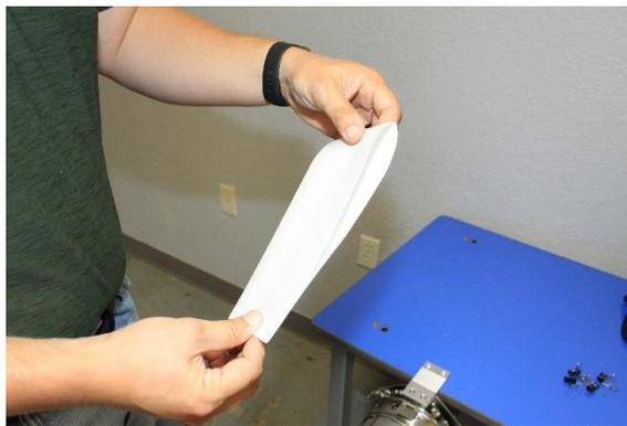
5. Unfold your cap backing and place it on your cap frame under the alignment tab. Be sure to line up the crease you made in step 3 with the center line in the alignment tab.
