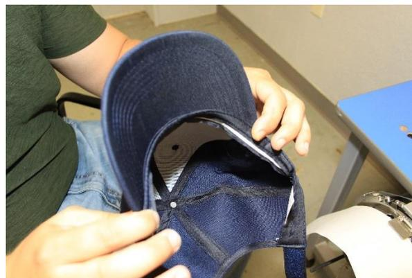
8. Place the cap onto the framing gauge on top of your backing with the sweat band going under the metal alignment tab.
