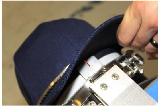
13. Hold down on the top of the cap and close the metal strap
