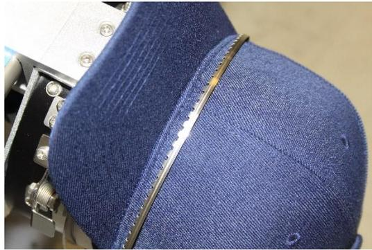
11. Loosely secure the strap on the right side of the cap frame
