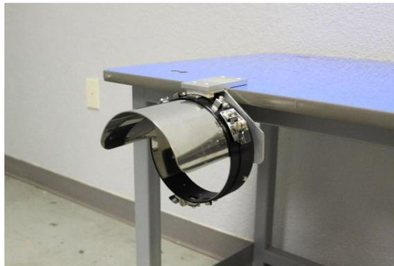
2. Load the cap frame onto the framing gauge by securing all three latches in place.
