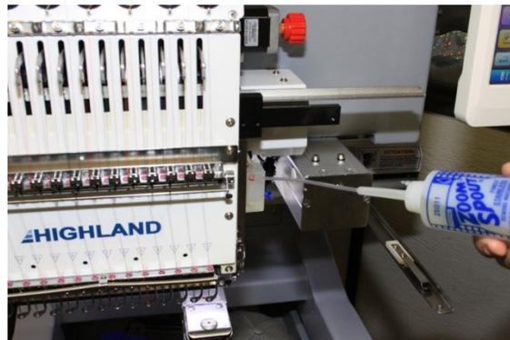
3. Inner portion of sewing head (Shafts and Connecting Rods)-One drop daily
