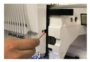
2. Put one drop of oil on the needle bar springs located behind the take up levers weekly
