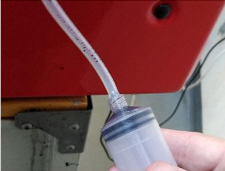
12. Detach syringe from waste ink line and place the line back in the waste container.
