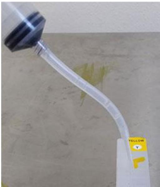
2. Use syringe to fill the cartridges.
