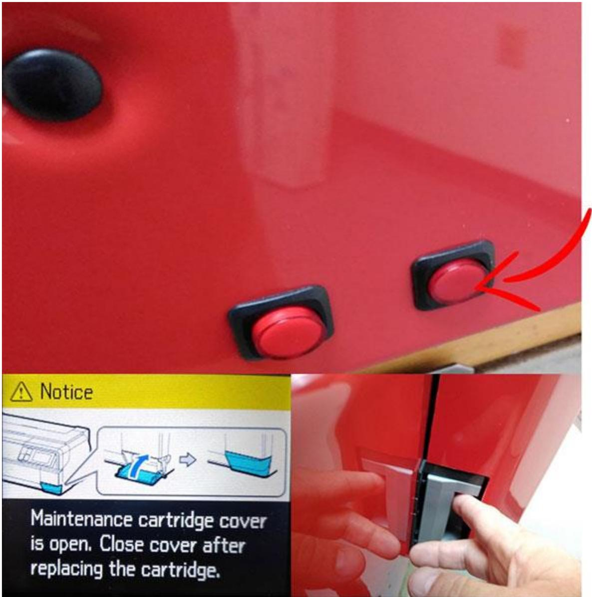
10. Press Cartridge Release button again. When it displays the Insert Maintenance Cartridge message, insert the new maintenance cartridge.
