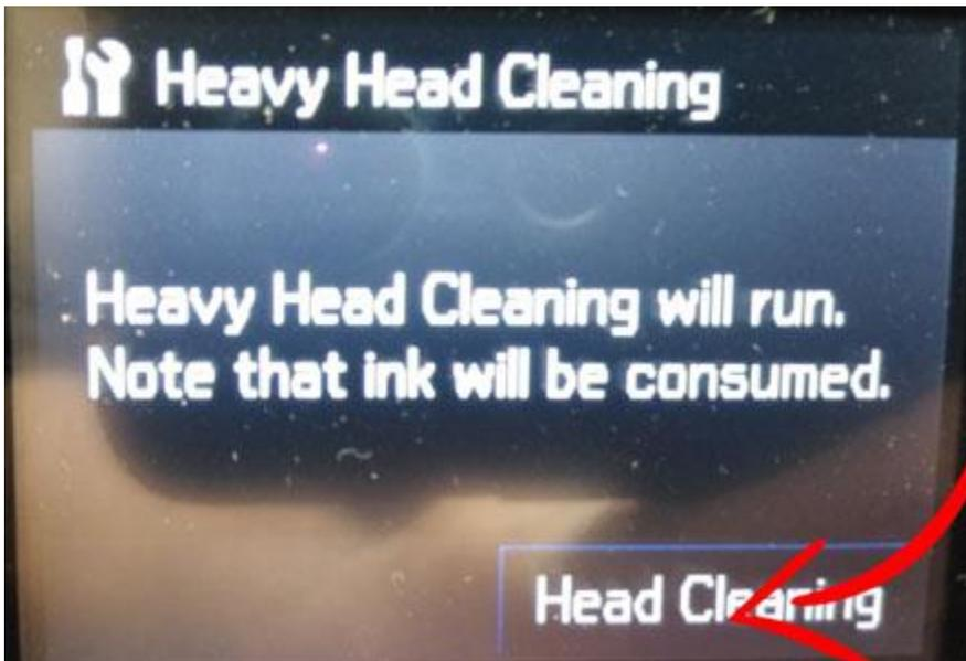
17. Once Heavy Head Cleaning is completed, repeat process until only clear liquid is coming through waste ink line.
