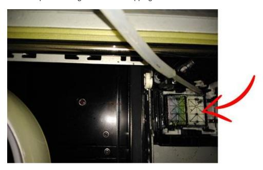
11. Clean with swab. Repeat until excess ink is removed. Using the same process, clean wiper blade.
