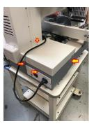
3. You will now see a silver cover held by 4 Phillips head screws, two which have ground wires secured to them. Please remove these screws, noting where the ground wires are connected (illustrated below).
