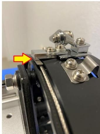
4. Tighten down the screws and make sure the metal tab is secure on the cable. Be sure to not over-tighten them as you can easily strip out the screw holes.
