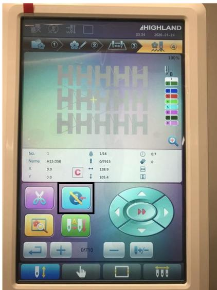
2. Press the 100 Button on the Control Panel (This will recycle the machine back to 100)
