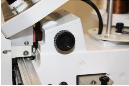
Turn the black knob on the right side of the machine until a number appears next to the needle on the top right of the control panel
