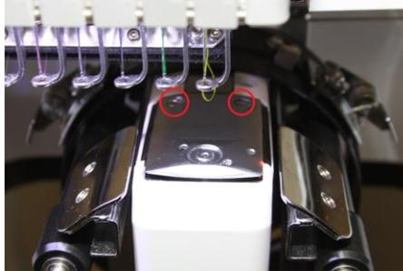
2. With the machine turned off, push the moveable knife back with your finger until it is tucked under the fixed knife
