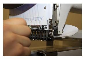
5. Place the needle alignment tool on the face of your needle. If it points to the right or to the left, loosen the needle clamp screw slightly and adjust the needle so that the eye of the needle is straight ahead. Your needle alignment tool will then point straight ahead as well.
