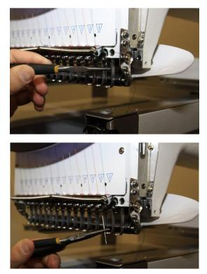
3. Using your needle nose pliers, insert the new needle so that the scarf is pointed towards the back of the machine
