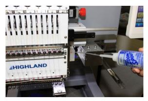
2. Inner portion of sewing head (Shafts and Connecting Rods)-1 drop on each point weekly.a. Move over to needle #1 and oil inside the hole on the silver plate
