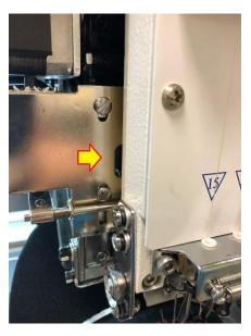
When oiling inside this hole, you are to hit the two points highlighted below:
