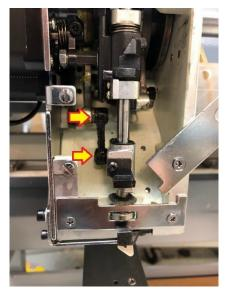
3. Needle Bars (springs behind take up levers)-1 drop on each needle bar spring weekly
