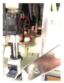
b. Move to needle #15 and oil inside the hole on the silver plate-1 drop on each point weekly
