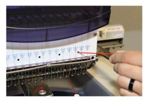
5. Hole on bed arm (small hole located behind the needle plate)- 2 drops, once daily
