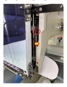
b. Move to needle #15 and oil the top of the reciprocator shaft
