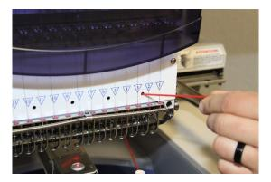
6. Hole on bed arm (small hole located behind the needle plate)- 2 drops, once daily
