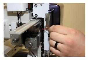
4. Needle Bars (springs behind take up levers)-1 drop on each needle bar spring weekly
