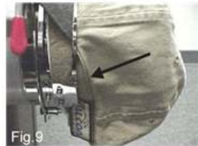
As mentioned before, this step is probably the most critical in framing a cap. If you do not keep the seams aligned with the teeth of the base and strap, your side embroideries will not sew out straight. That is, they will tilt at an angle to the seam of the cap. Figure 9 shows the seam and strap incorrectly aligned.
